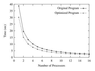
Figure 7. The computation time before/after the optimization.
